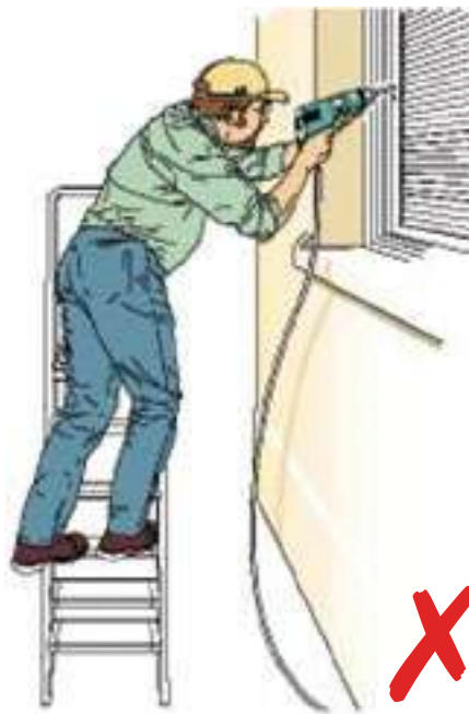
Figure 31: Incorrect – steps are side-on to work activity.
