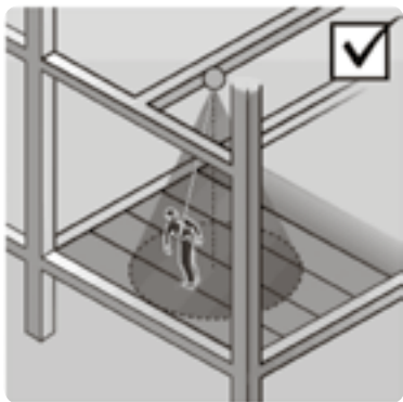
Figure 14: Working within an arc below the inertia reel.
